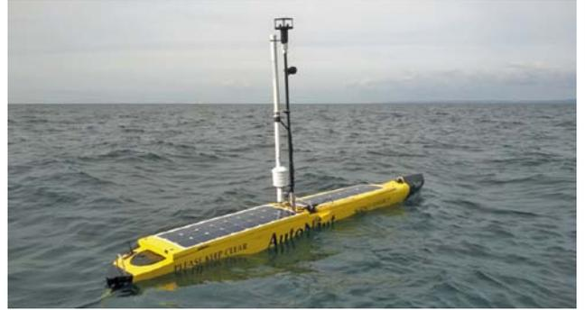
AutoNaut showing the installation of the ‘AMOS’ met sensors. Also on the mast are a camera and WiFi antenna to trial transmission of HD photos and video
